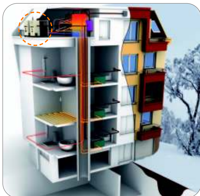
Example of GAHP-AR application in winter and summer operation for radiant panels, fan coils, indirect production of DHW.
