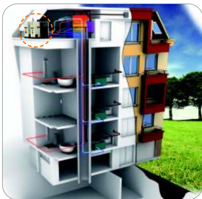
Example of GA-HR application with reversible GAHP-AR heat pump in summer operation for fan coils and indirect DHW production.
