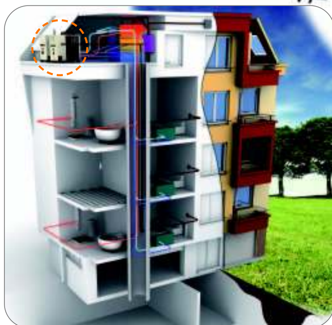
Example of GAHP-AR application in winter and summer operation for radiant panels, fan coils, indirect production of DHW.
